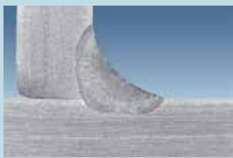
WIG DC, Argon, v_s = 13 \text{ cm/min}
