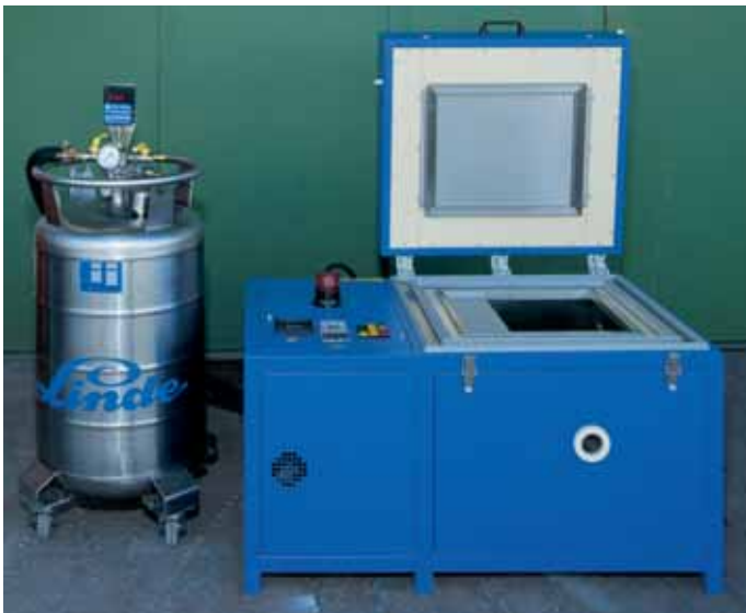
Figure 15: Liquid Nitrogen Stored in a Pallet Tank Holds Typically 600 Liters (300 Gallons) of LIN
