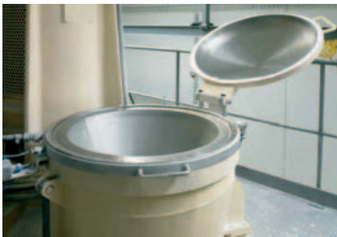
Fig. 11: N2LOCK® inert gas lock integrated into the charging port of a mixer
