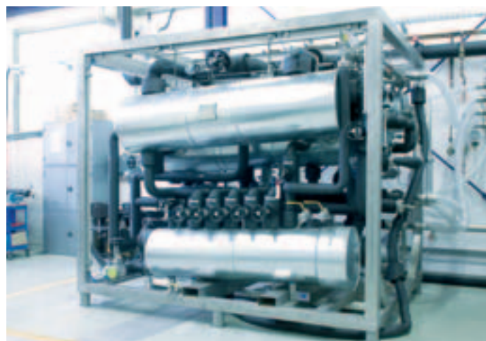
Fig. 14: Test unit for hydrocarbon recovery by three-stage cryocondensation
