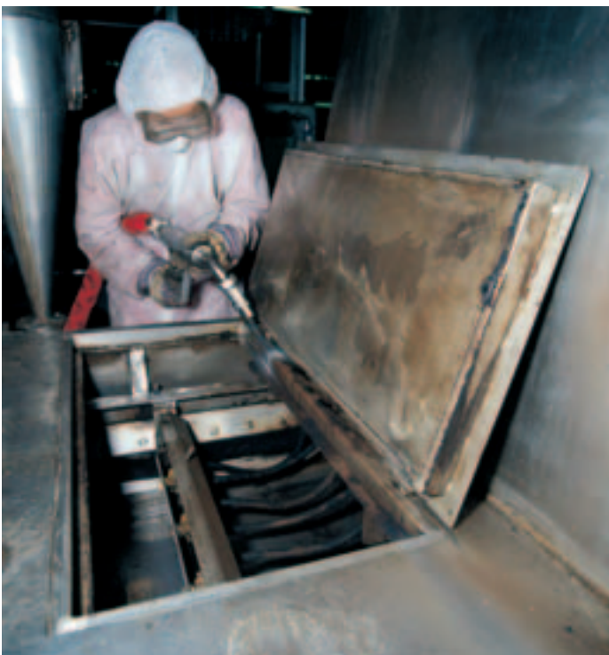
Fig. 19: Cleaning with the CRYOCLEAN® process in a coffee processing plant
