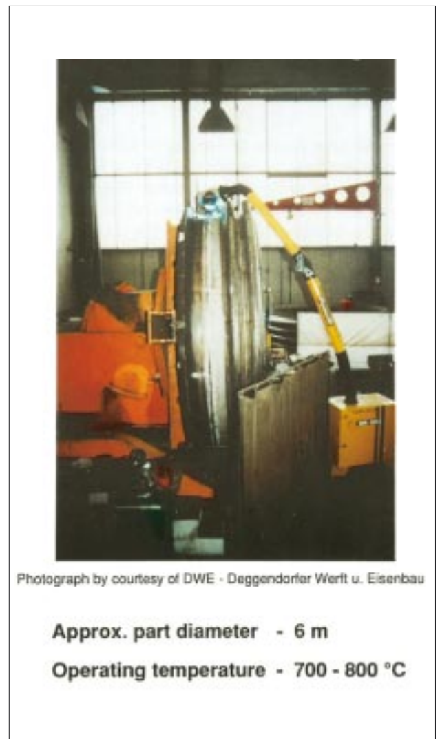
Fig. 16 MAG welding of nickel base alloys Exhaust gas diffuser for gas turbines
